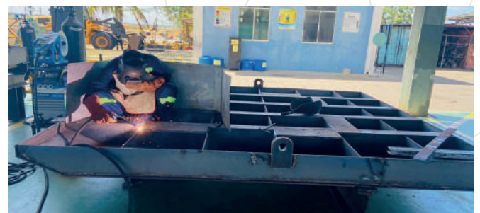
A fender - plate undergoing repairs at the workshop.
